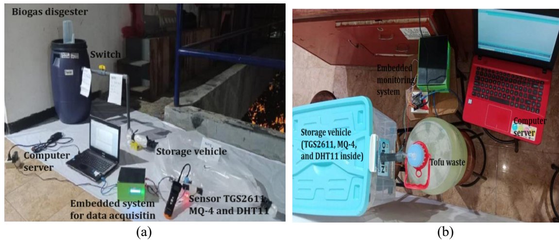
Figure 6. Monitoring of methane gas. (a) biogas digesters, (b) tofu waste storage vehicles.
